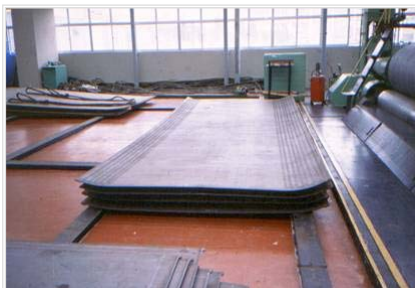
Crimping of plate edges
