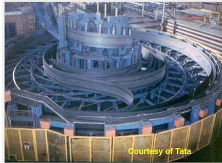
Coil accumulator
